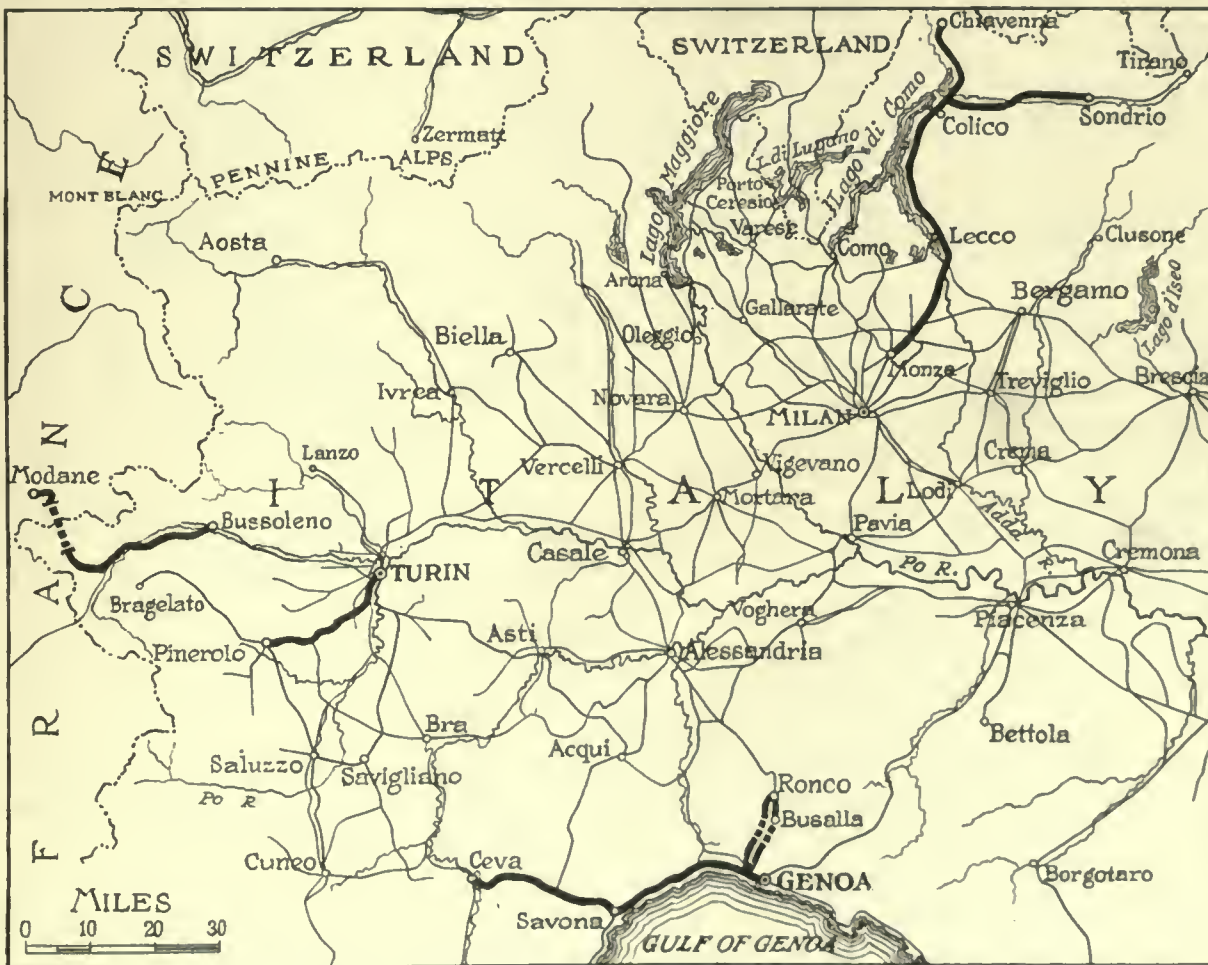
FIG. 479. ITALIAN TRUNK LINE ELECTRIFICATIONS
